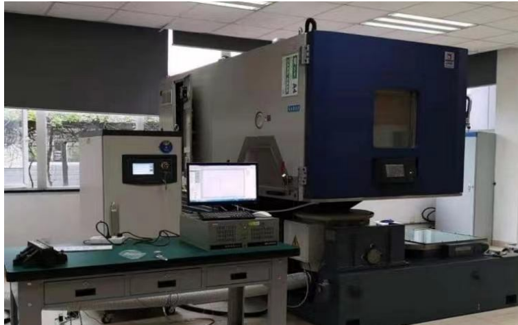
Figure 1. Temperature rise test device of single battery
