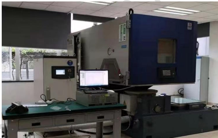
Figure 1. Temperature rise test device of single battery
