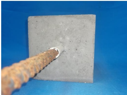
Fig. 2 .Pull Out Damage
