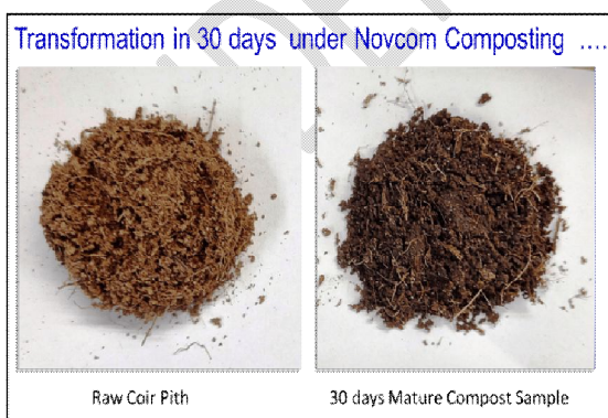
Pic. 15 : Transformation of raw coir pith to mature compost in 30 days under Novcom Composting Technology.
