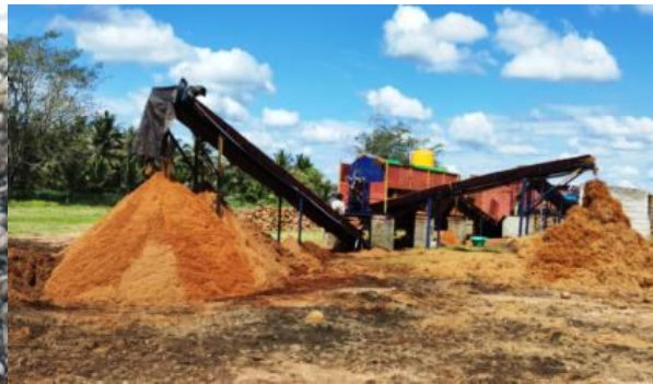
Pic. 2 : Coir factory for extracting coir fibre and coir husk.
