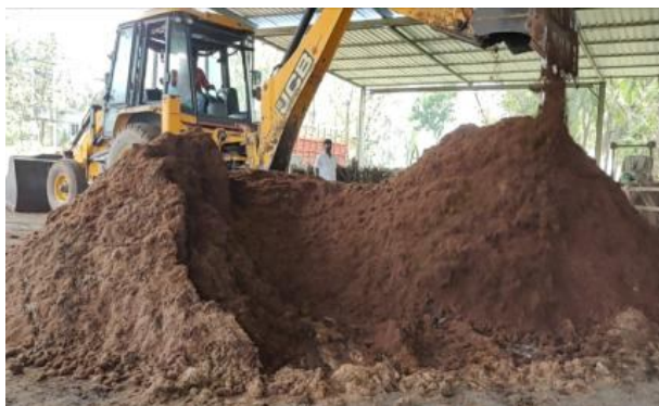
Pic. 7 : Mixing of raw coir pith with cow dung slurry at Mandya, Karnataka
