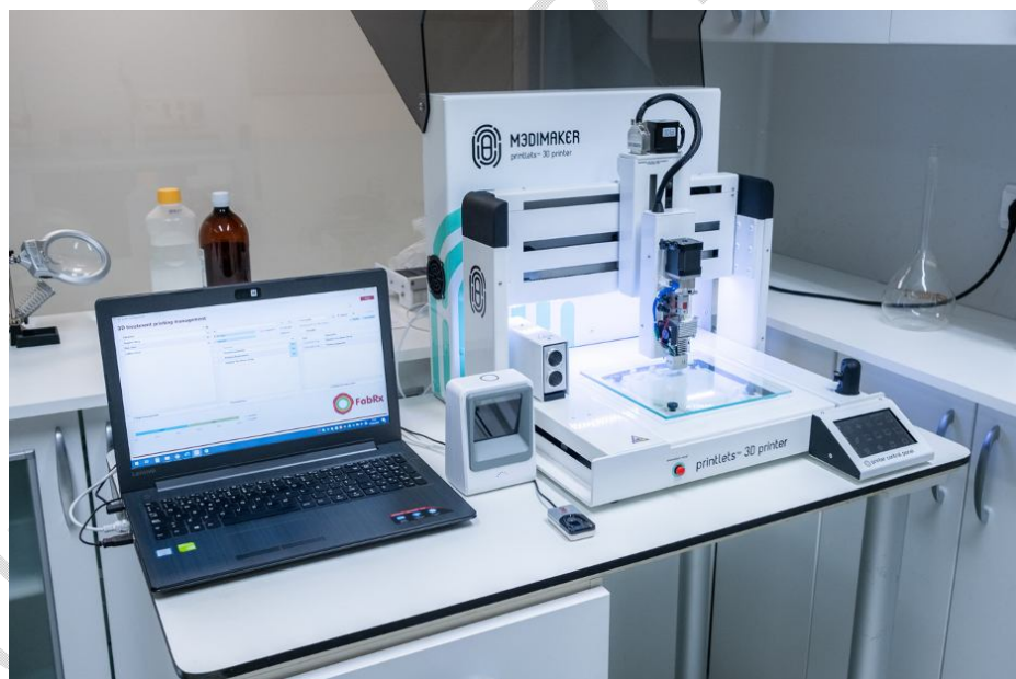
Figure.3 FabRx's pharmaceutical 3D printer for personalized medicines, M3DIMAKER (21)
