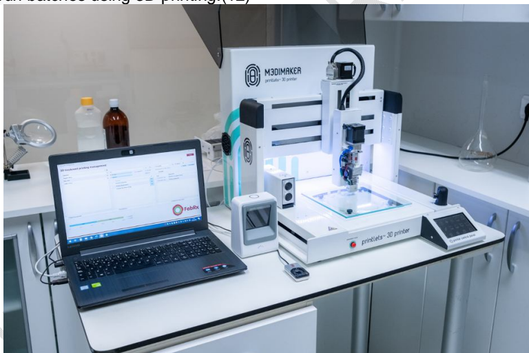
Figure.3 FabRx's pharmaceutical 3D printer for personalised medicines, M3DIMAKER
