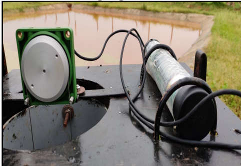
Plate 2b: Close view of thalimede data encoder and data logger used in the study area
