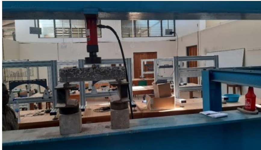
Figure 5: Flexural test on concrete prism.
