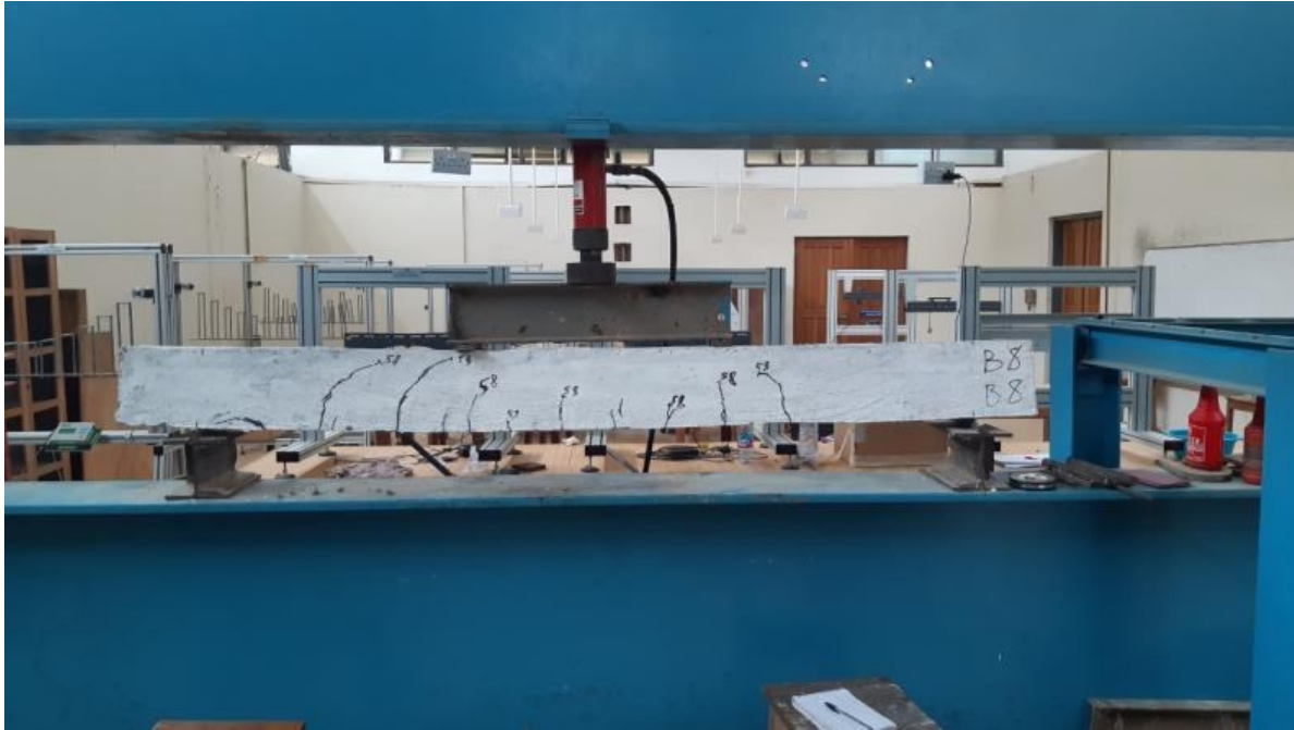
Figure 16: Beam 8 failure mode
