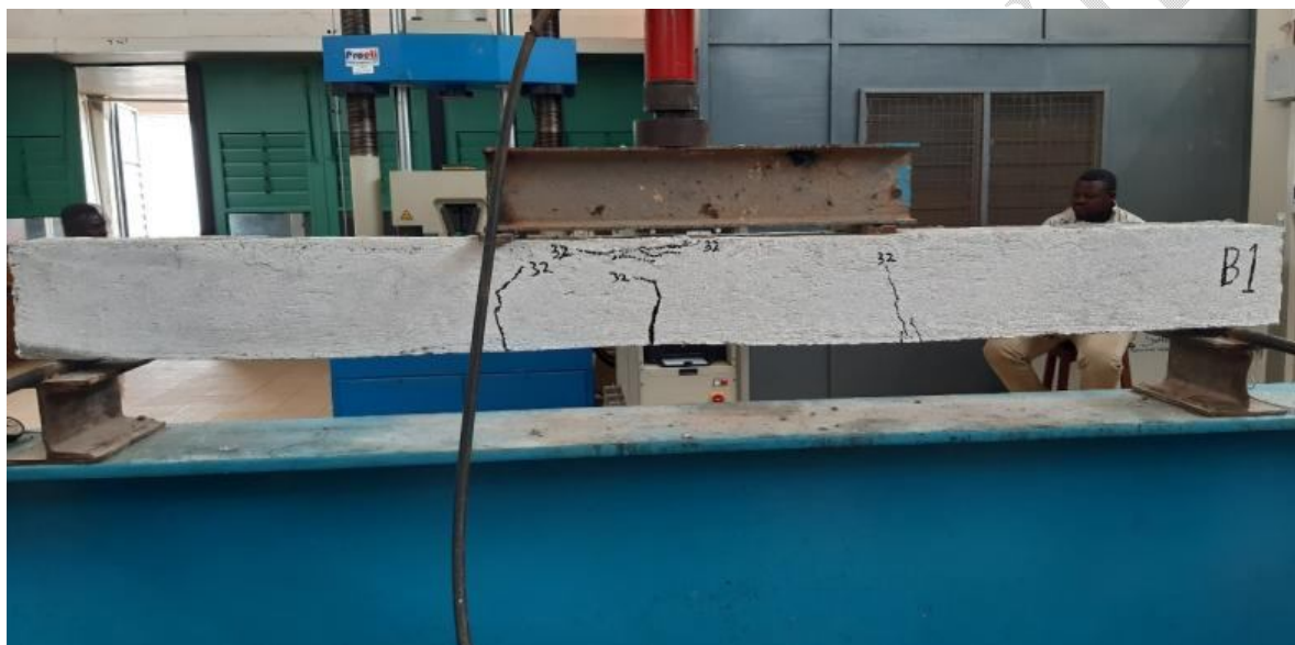
Figure 9: Beam 1 at failure
