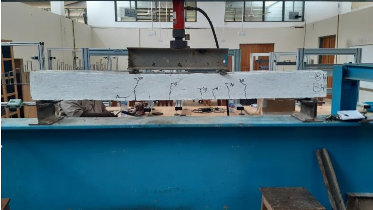
Figure 12: Beam 4 failure mode
