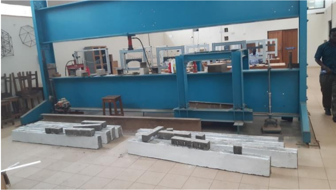
Figure 6: Concrete beams ready for testing
