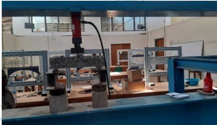
Figure 5: Flexural test on concrete prism.
