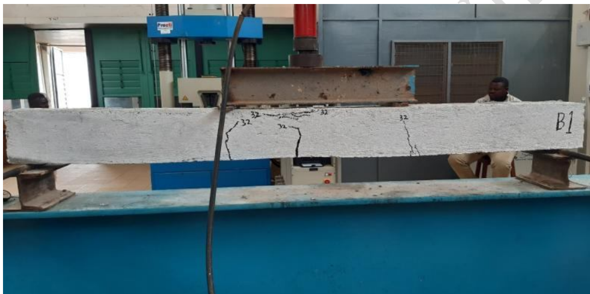
Figure 9: Beam 1 at failure
