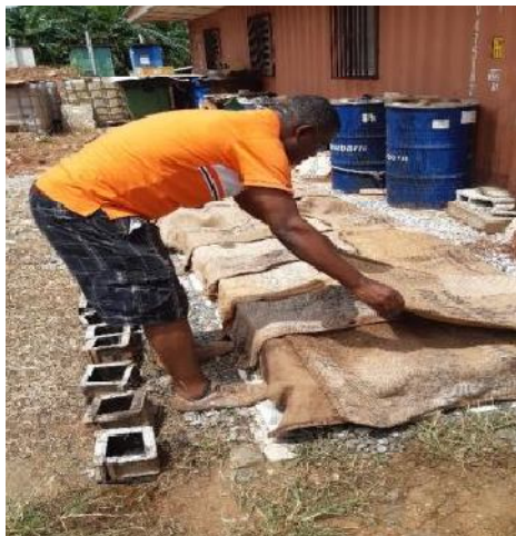
Figure 3: Curing of specimens Beams
