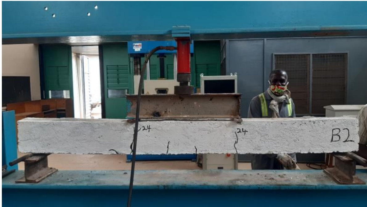
Figure 10: Beam 2 at failure
