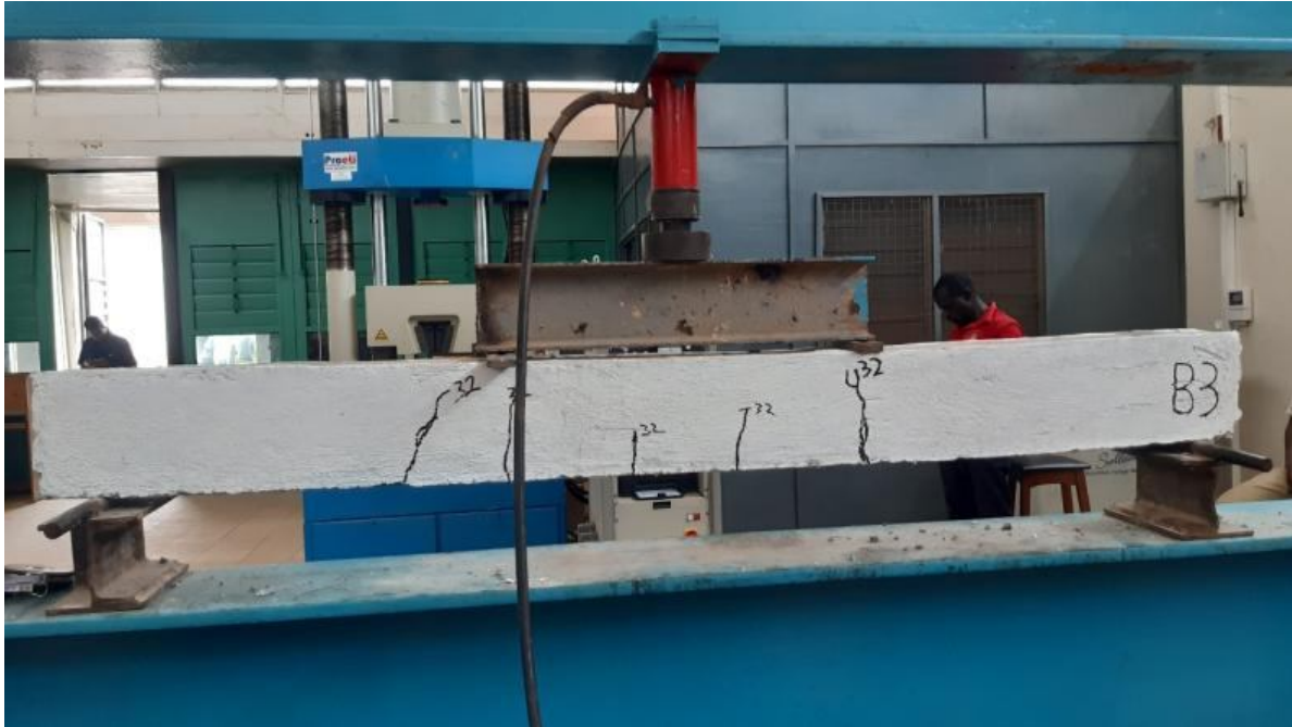
Figure 11: Beam 3 failure mode
