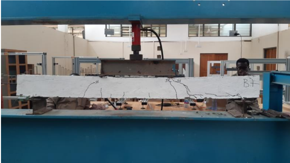
Figure 15: Beam 7 failure mode
