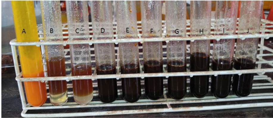
Image 1. Effect of chemical bleaching on the colour of unadulterated and adulterated palm oil samples
