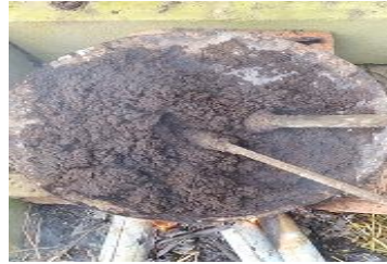
Fig-1: Plastic and sand mix are burnt
