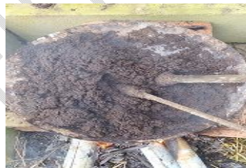
Fig-1: Plastic and sand mix are burnt
