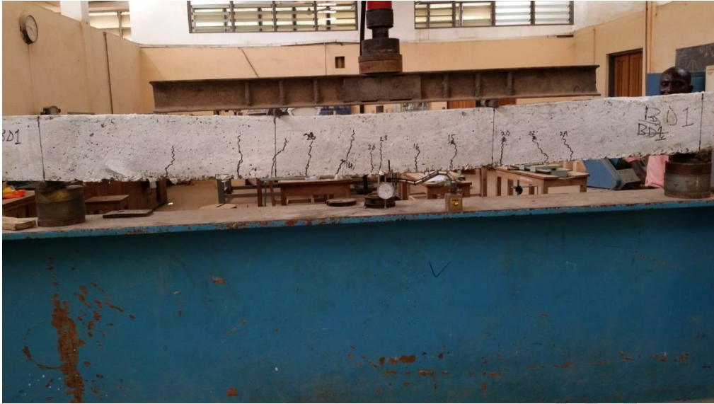
Figure 7: Crack propagation and characteristics of the 1.0% fibre concrete
