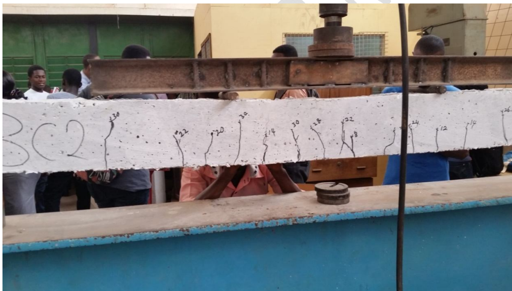
Figure 6: Crack propagation and characteristics of the 0.5% fibre concrete
