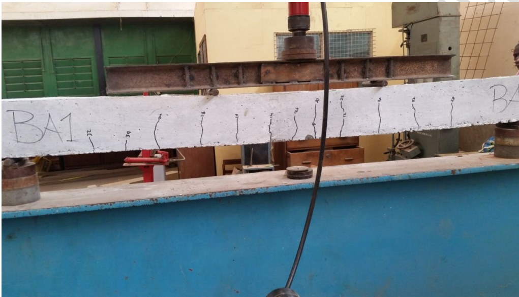
Figure 4: Crack propagation of the control specimen
