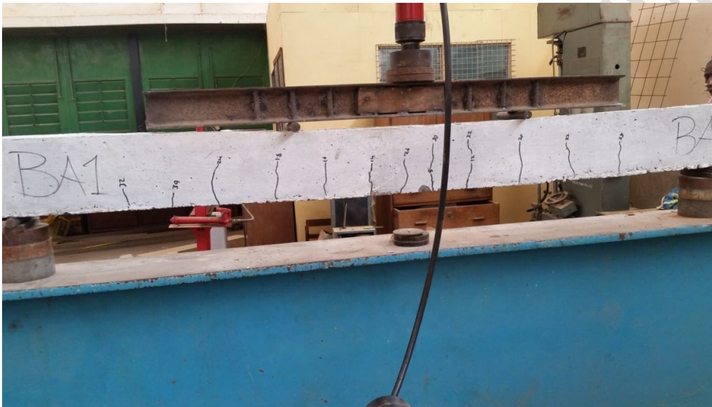
Figure 4: Crack propagation of the control specimen
