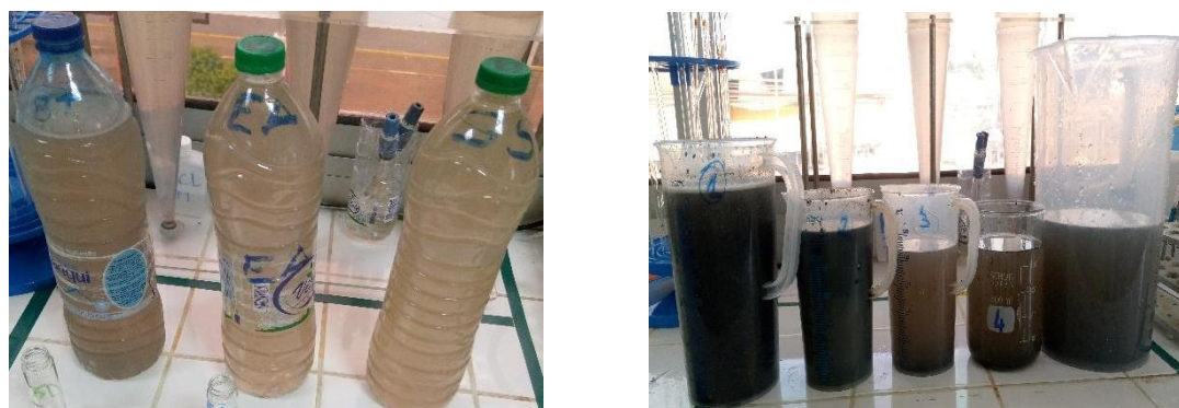
Figure 1: Samples of wastewater (A) taken at the entrance to the WWTP in the buffer basin (BT), the anaerobic effluent channel (EA) and at the WWTP outlet (SS) and anaerobic sludge from the UASB reactor (B).
