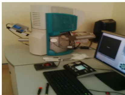
Fig. 3. Scanning Electron Microscope (BRUKER 125ev) used for the SEM Analysis.
