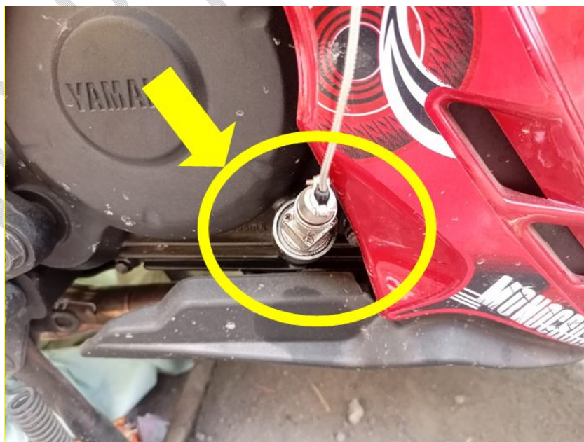
Figure 8 Potitioning of Thermocouple
