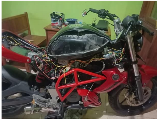
Figure 6 Electronic circuit placement
