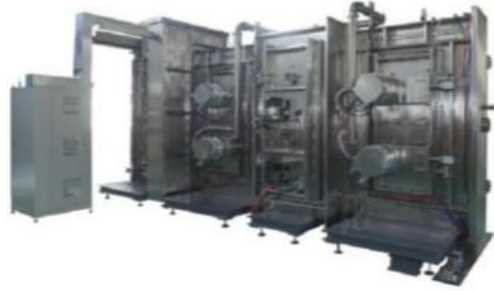
Fig.3.Metal sheet surface coating equipment
