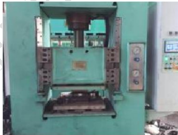
Fig.5.Metal bipolar plate stamping machine
