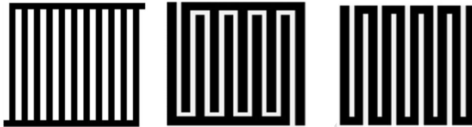
Figure 2 (a) Parallel flow field (b) Alternating finger flow field (c) Serpentine flow field
