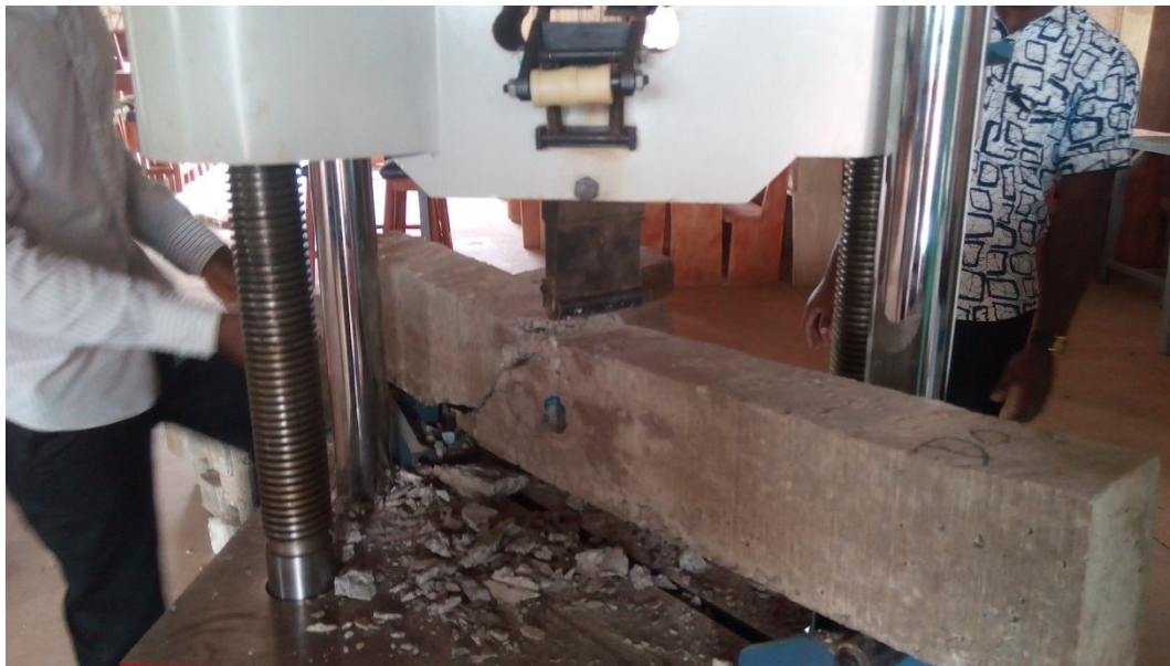
Plate 3: Mode of Failure of Experimental Beam TIII
