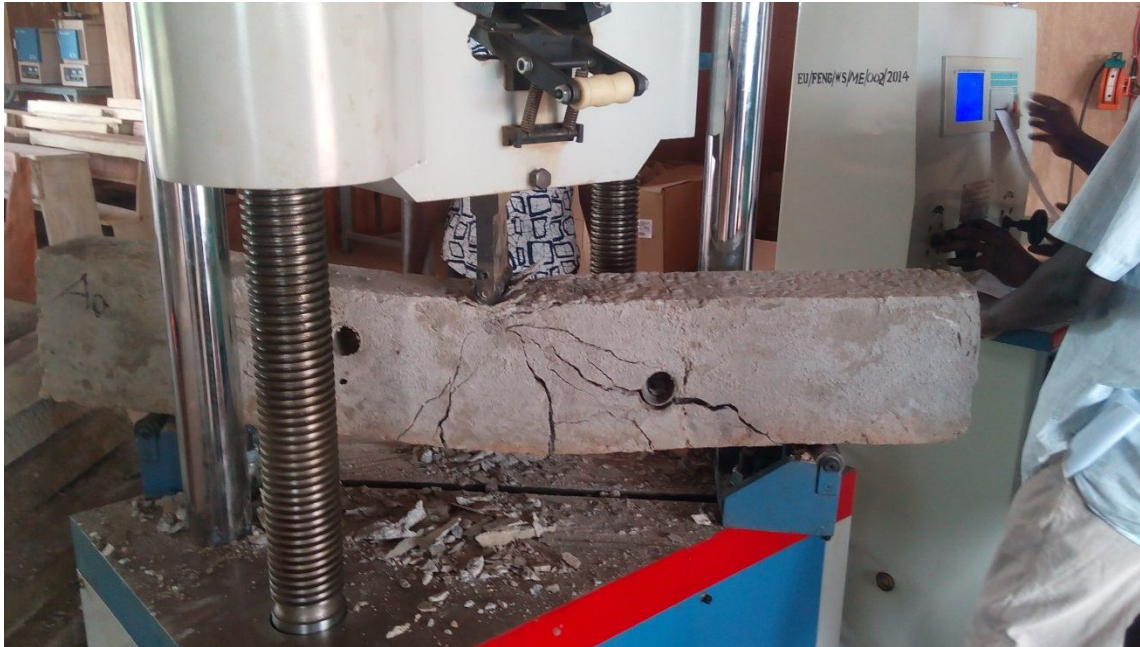
Plate 4: Mode of Failure of Experimental Beam TIV
