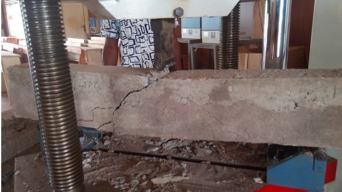
Plate 1: Mode of Failure of Control Beam TI
