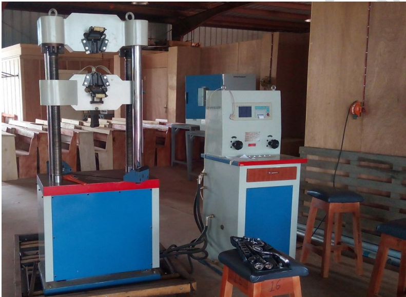
Plate 2: The Universal Testing Machine Setup
