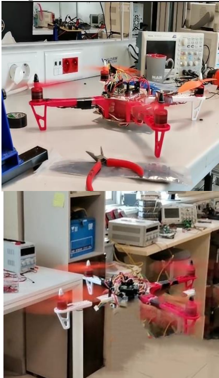
Fig. 26. The quadcopter flight test
