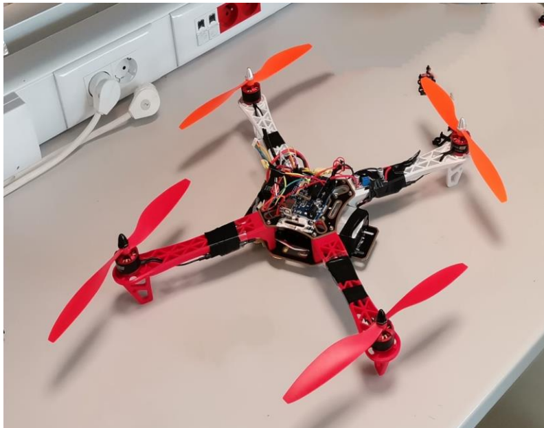
Fig. 16. The Quadcopter Hardware Implementation
