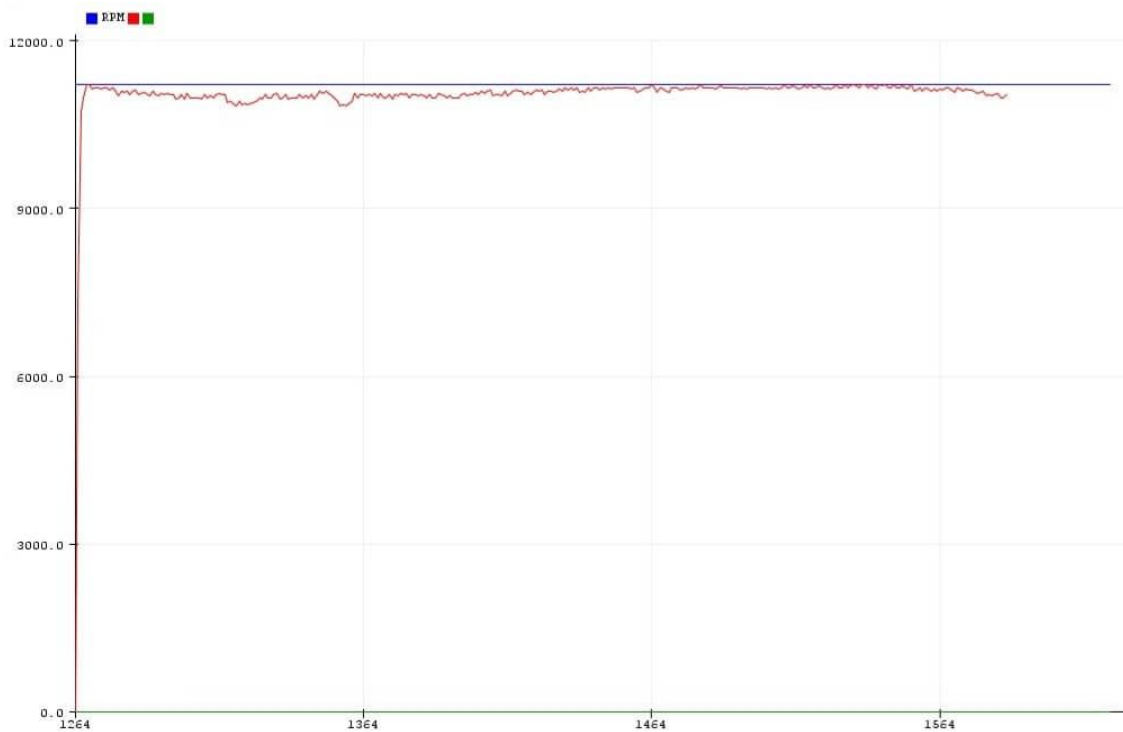
Fig 8: Motor response when sending command the number 1 or 2 or 3 (11228 rpm)
