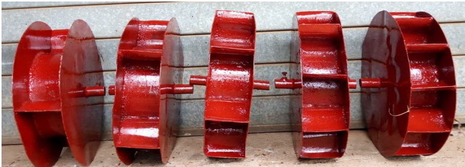
Fig.1. Turbine Runners with Splined Blades used for the study
