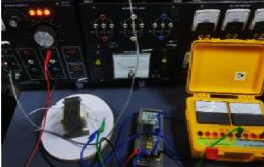
Fig. 8. Practical setup for the performance test of the designed 1- \phi transformer
