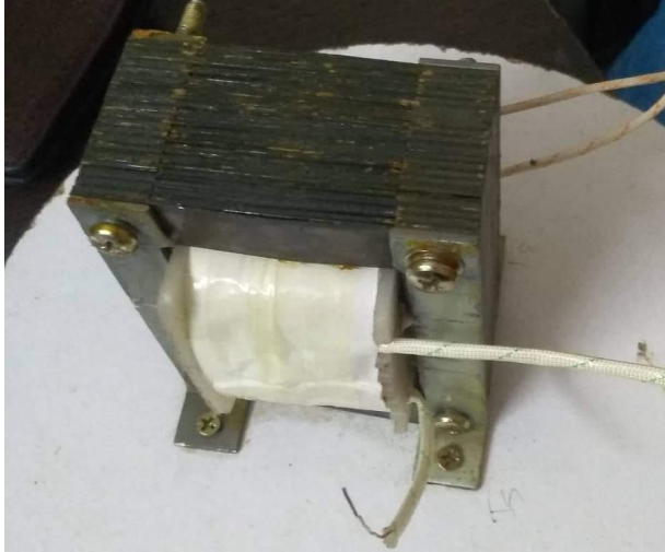
Fig.5.Manufactured single-phase transformer on the base
