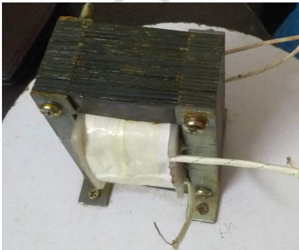
Fig. 5. Manufactured single-phase transformer on the base
