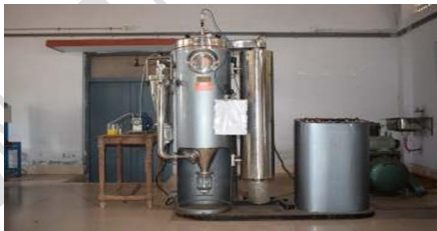
Plate 1: Laboratory model pilot scale spray dryer
