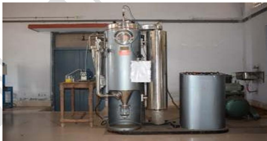
Plate 1: Laboratory model pilot scale spray dryer
