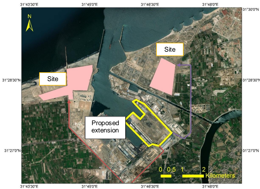
Fig 21. Two sites proposed to dispose sediment dredged from the extension harbor basin (project area). Site #1 is identified in this study as a low-lying area suitable for land filling whereas Site #2 has been previously used for dumping sediment excavated from the navigation canal connecting between the main basin and the Damietta Nile branch whereas. General pathways connecting between the proposed dumping sites and the excavated basin are also denoted as lines.
