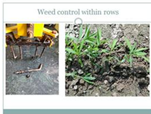
Photo 5. Weed control “ within rows ” in sunnhemp by Agricultural Weeder with Nail assembly opening its central nail.
