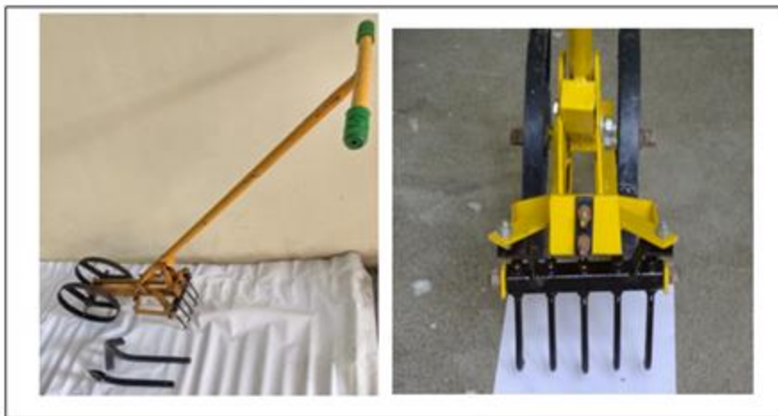
Photo 1. Agricultural weeder with nail assembly, Design registration no. 289754 in class 15-03, dt. 13-09-2019, Patent Office Kolkata, Govt. of India
