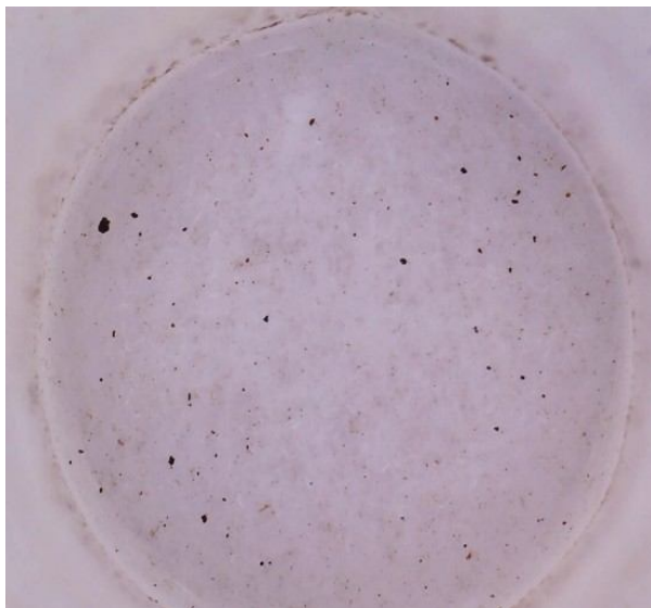
Figure 4: 1000 particles of black carbon particles per litre of water; collected in the Equatorial Atlantic Ocean. Ref18
