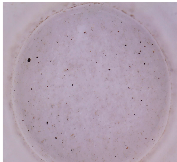
Figure 4: 1000 particles of black carbon particles per litre of water; collected in the Equatorial Atlantic Ocean. Source: Goes Foundation
