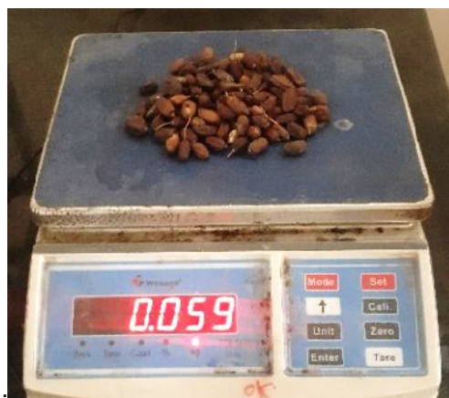
Fig. 1: Weighing of 100 neem seed using digital weighing balance.
