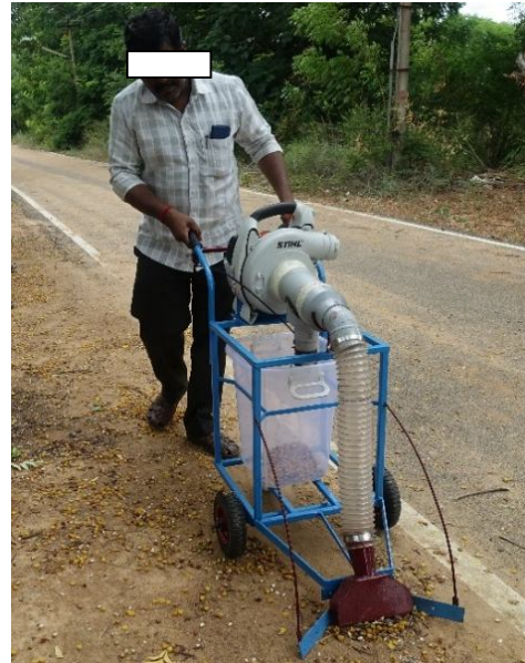
Fig. 5(b). Operational view of the ground collection machine for neem fruit.
