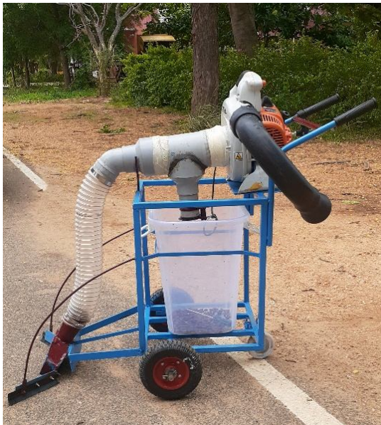
Fig. 5(a). Ground collection machine for Neem fruit.
