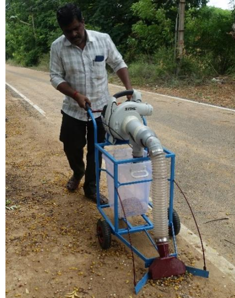
Fig. 5(b). Collection of neem fruit by the developed prototype
