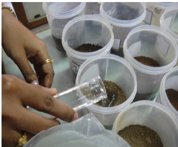
Addition of water to maintain 75% WHC
