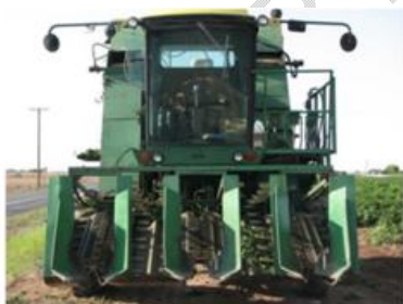
Fig. 1. Massey's three-row self-propelled pepper harvester
