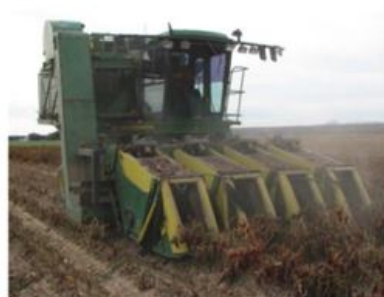
Fig. 2. McClendon four-row self-extracting dry red pepper harvester
