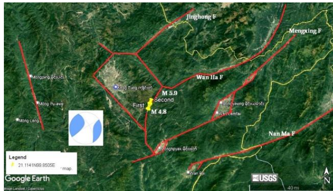
Fig.3. Google Earth map showing location of two earthquakes M 4.8 and M 5.9 on Wan Ha Fault with focal mechanism solution of earthquake.
