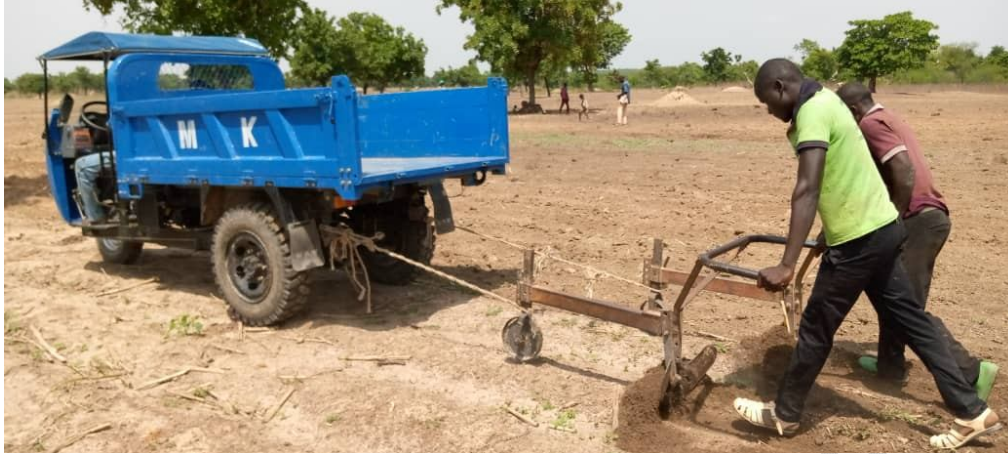
Pict 1: Motorized plow with a trike used for tilling Source: Author photo, 2020
