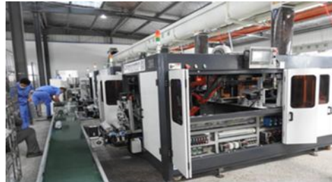
Fig.1. The automatic bacillus bagging machine
