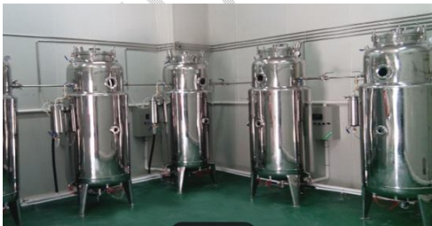
Fig. 5. The bit sterilization fermenter
