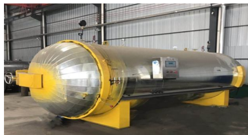
Fig. 2. The Double-door autoclave steam sterilizer
