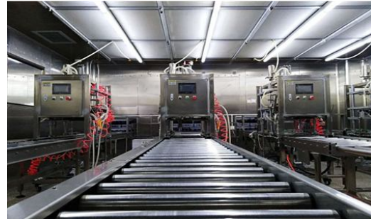
Fig.3.The automatic bacillus bagging machine
