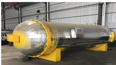
Fig. 2. The Double-door autoclave steam sterilizer
