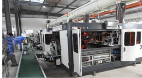
Fig. 1. The automatic bacillus bagging machine
