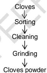
Fig. 4: Flow chart for the preparation of cloves powder Source: Kumar and Tanwar (2011) [10]
