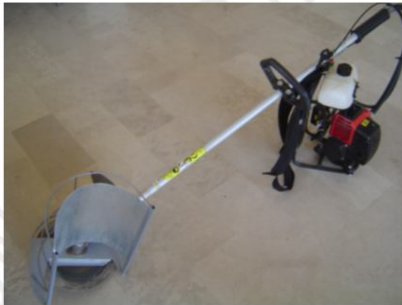
Fig. 3 Portable mechanical brush-cutter
