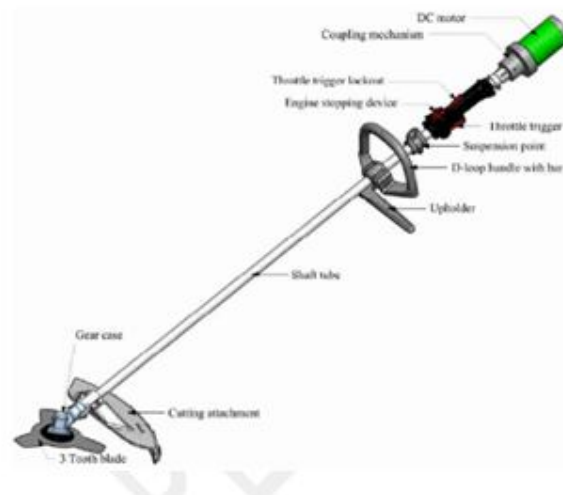
Fig. 6 Electric operated three tooth blade bush cutter
