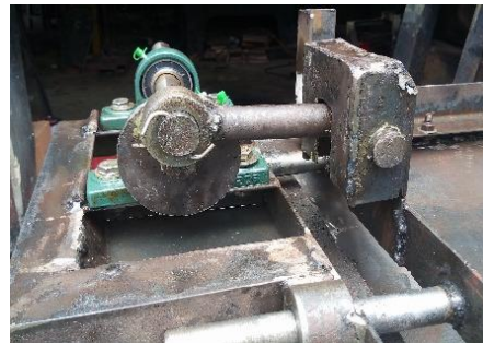
Fig. 6: Slider-Crank of the Developed Machine
