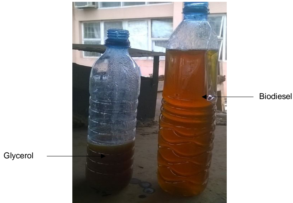
Figure 4 : Glycerol and Biodiesel in container after separating process.
