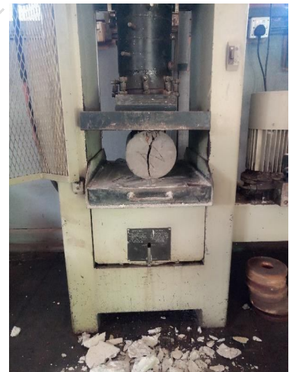
(c) Load applied to cylinder until failure
