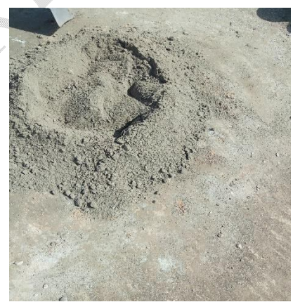
(c) Mixture of cement, recycled glass powder and fine aggregates
